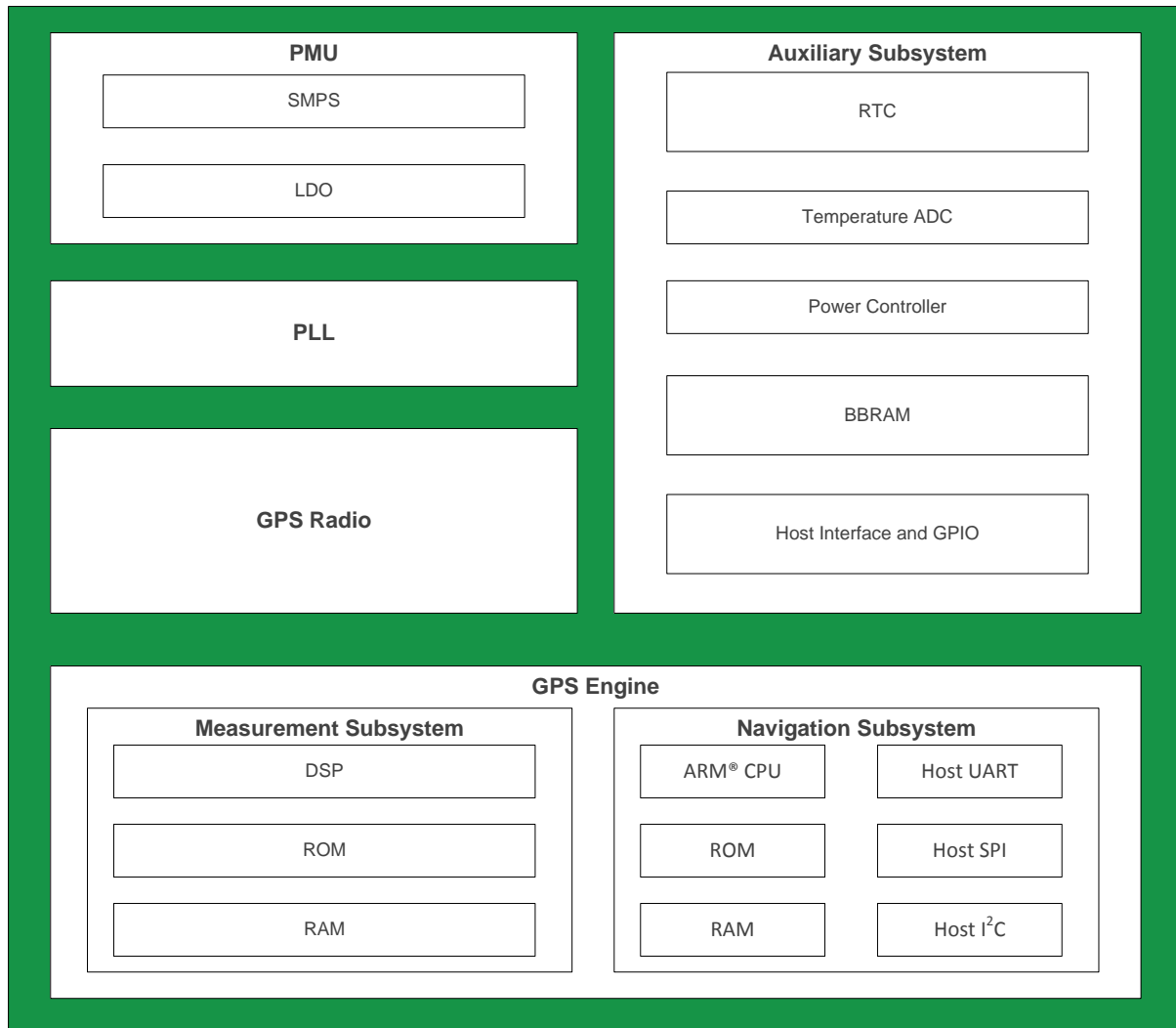
FIGURE 2 – SiRFstarIV™ GSD4e GPS SoC BLOCK DIAGRAM
