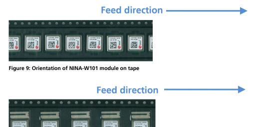
Figure 10: Orientation of NINA-W102 module on tape
