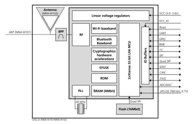
Figure 1: Block diagram of NINA-W10 series
