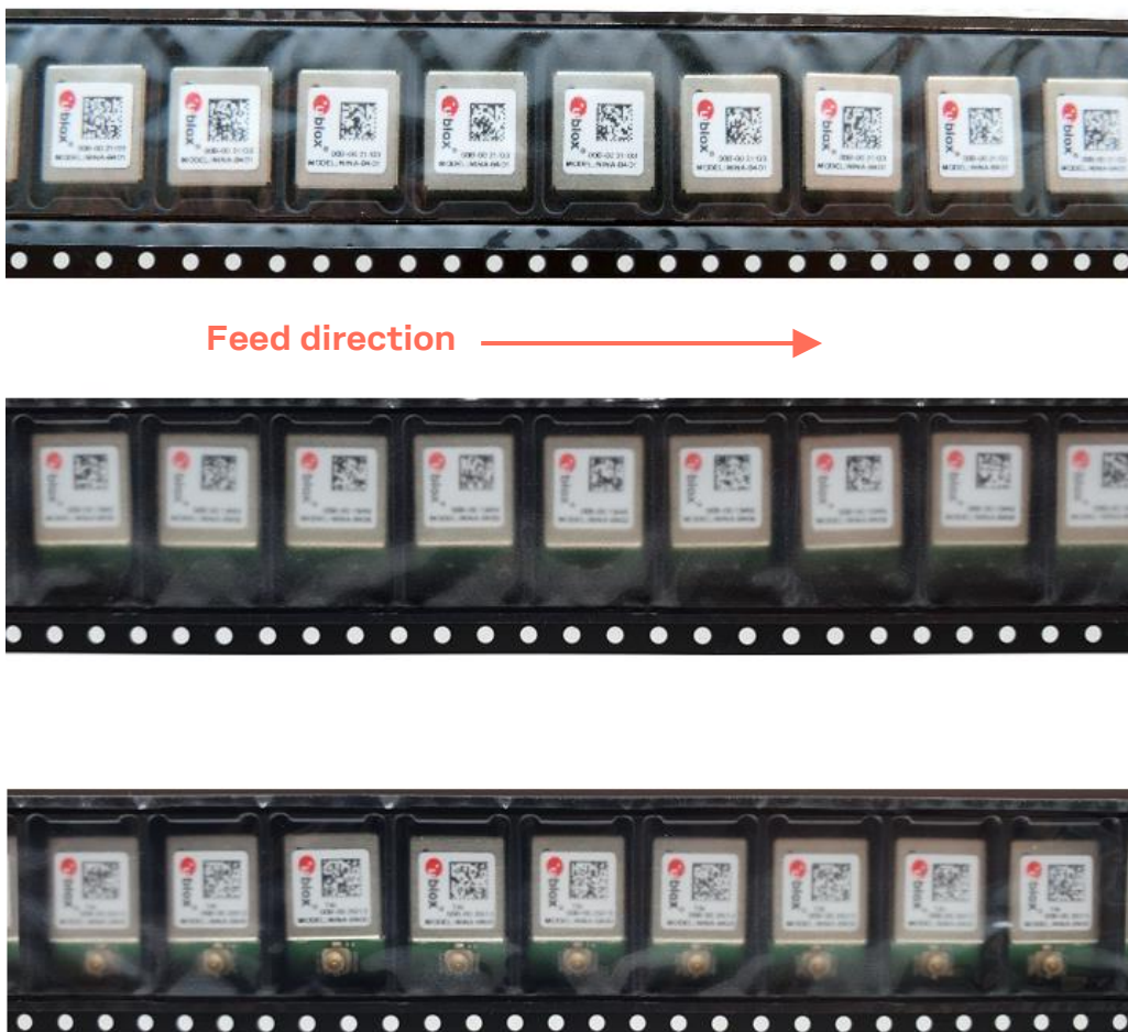
Figure 9: Orientation of NINA-B41 modules on tape
