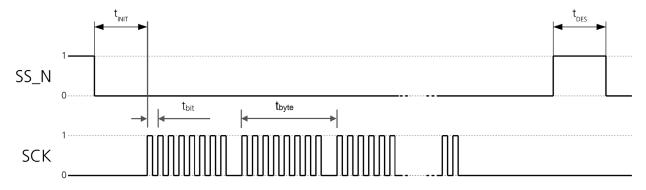
Figure 5: SPI timing diagram
