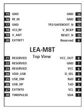
Figure 4: LEA-M8T pin assignment
