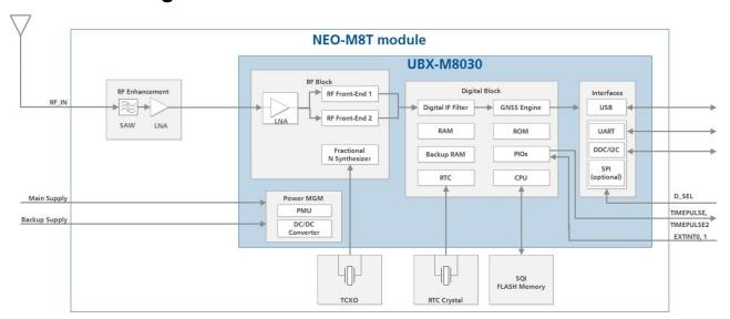
Figure 1: NEO-M8T block diagram
