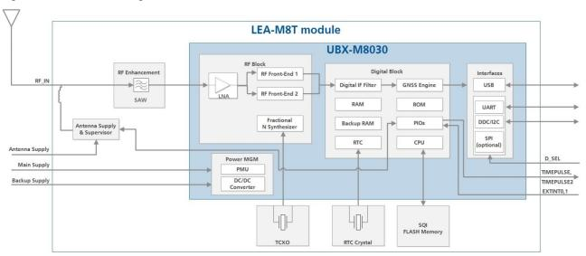
Figure 2: LEA-M8T block diagram
