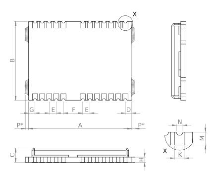
Figure 6: NEO-M8T mechanical drawing
