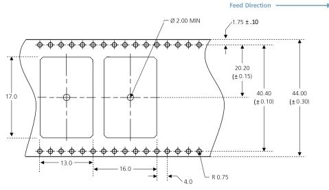
Figure 8: Dimensions and orientation for NEO-M8T modules on tape
