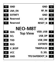
Figure 3: NEO-M8T pin assignment
