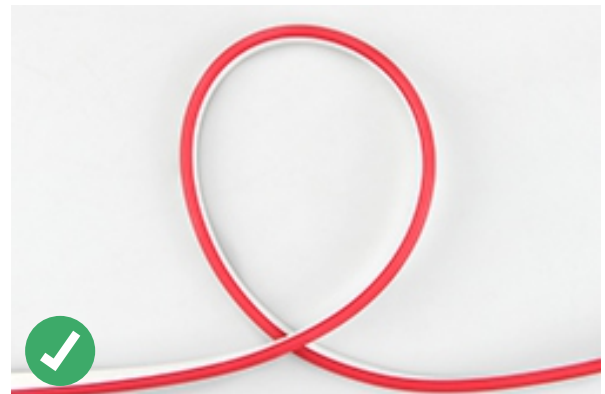
Lighting surface upwards and the strip can be bent to right or left naturally, The minimum bending diameter is 100mm
