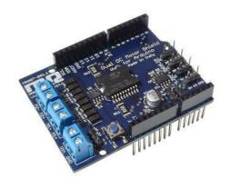
The *Dual DC Motor Shield* is a shield that has been projected to enable an Arduino board to drive two brushed DC motors or one 4-wire two-phase stepper motor, controlling the speed and direction of each one independently.
