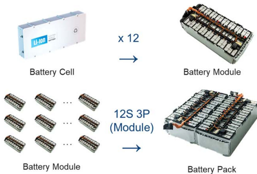
Figure 1 – Battery Pack Structure Example (Image)
