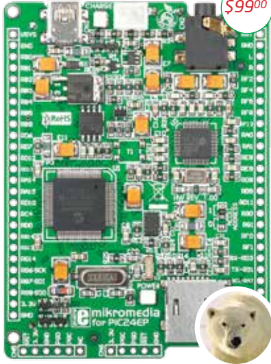
mikromedia for PIC24EP (features PIC24EP512GU810)
