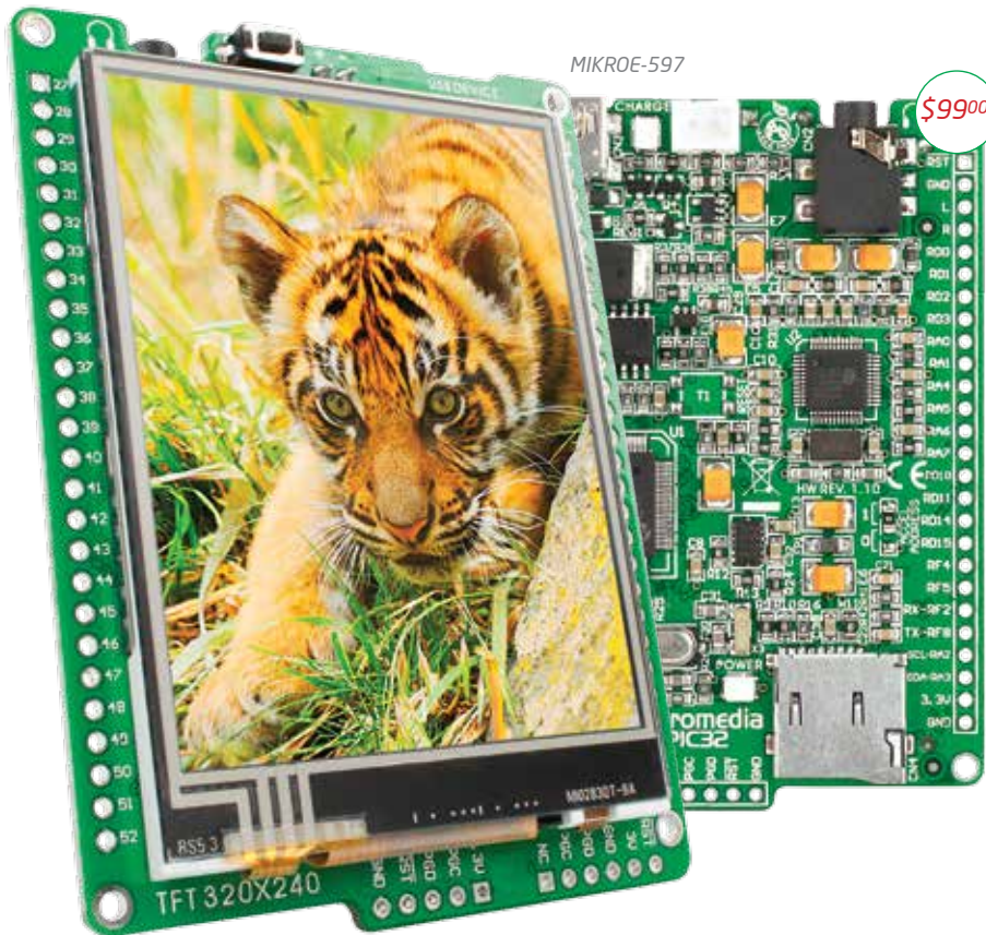
mikromedia for PIC32 (features PIC32MX460F512L)
