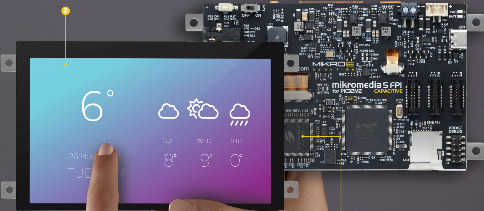
Figure 10: Display and SSD1963 view
