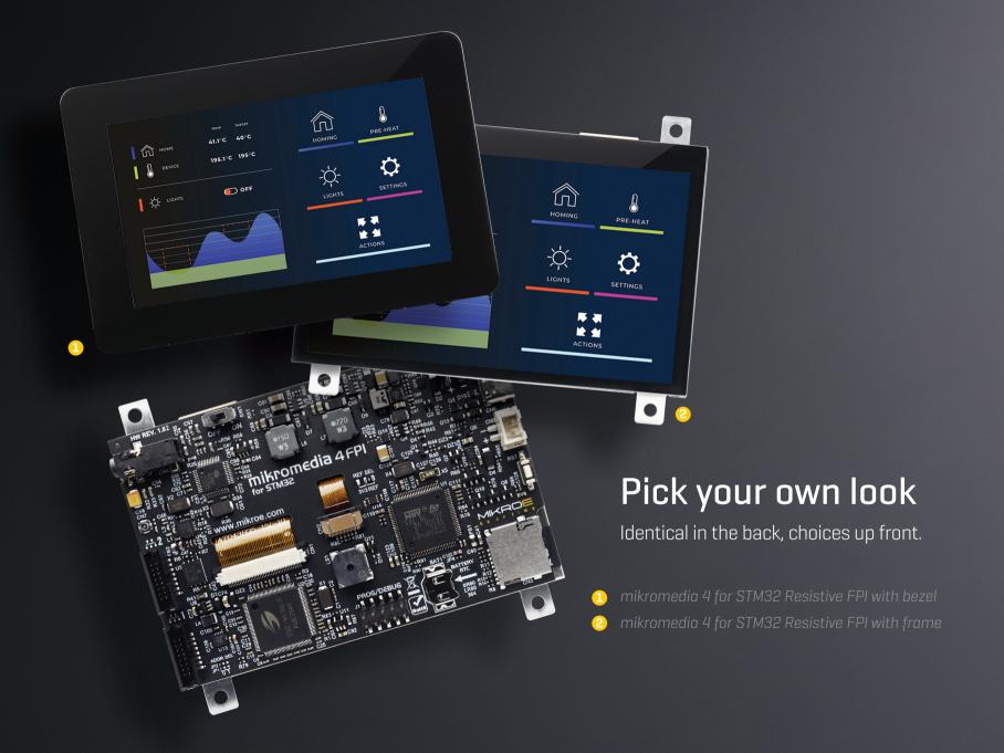
mikromedia 4 for STM32 RESISITVE FPI is a compact development board designed as a complete solution for the rapid development of multimedia and GUI-centric applications. By featuring a 4.3" resisitve touch screen driven by the powerful graphics controller that can display the 24-bit color palette (16.7 million colors), along with a DSP-powered embedded sound CODEC IC, represents a perfect solution for any type of multimedia application.
