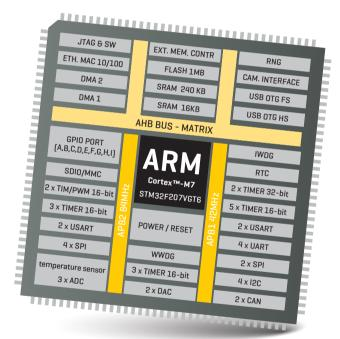
Figure 2: STM32F207VGT6 MCU block schematic
