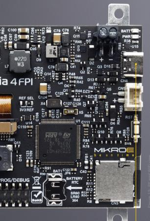
Along the SPI lines, it uses additional GPIO pins for the SPI Chip Select, Chip Enable, and for the interrupt. The RF section of the mikromedia 4 FPI also features a small chip antenna as well as SMA connector for external antenna.
