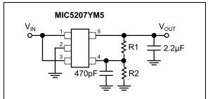
FIGURE 4-3: Ultra-Low-Noise Adjustable-Voltage Application.
