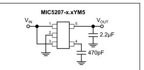
FIGURE 4-1: Ultra-Low-Noise Fixed-Voltage Application.
