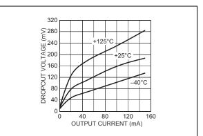
FIGURE 2-12: Dropout Voltage vs. Output Current.
