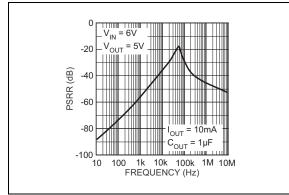
FIGURE 2-7: Power Supply Rejection Ratio.
