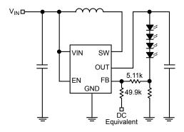
Figure 2. Continuous Dimming
