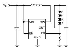
Figure 3. MLF® Package OVP Circuit
