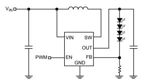
Figure 1. PWM Dimming Method
