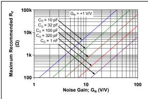
**FIGURE 4-12:** Maximum Recommended  $R_F$  vs. Gain.
