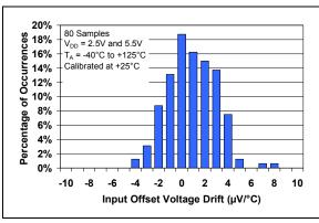
FIGURE 2-2: Input Offset Voltage Drift.
