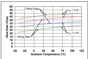
FIGURE 2-42: Slew Rate vs. Ambient Temperature.
