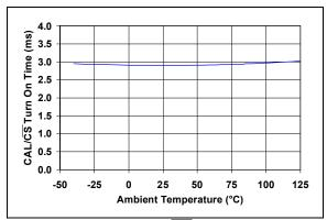
**FIGURE 2-48:** CAL\overline{\text{CS}} Turn-On Time vs. Ambient Temperature.
