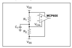
**FIGURE 4-2:** Setting  $V_{CM}$  with External Resistors.
