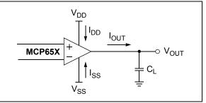
**FIGURE 4-8:** Diagram for Capacitive Load Power Calculations.
