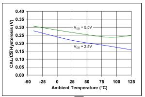
**FIGURE 2-47:** CAL/CS Hysteresis vs. Ambient Temperature.
