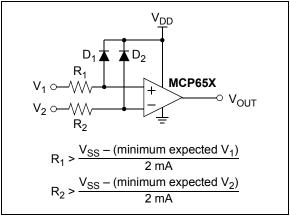
FIGURE 4-4: Protecting the Analog Inputs.
