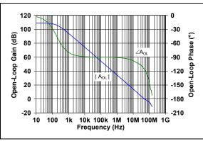
FIGURE 2-25: Open-Loop Gain vs. Frequency.
