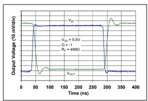
**FIGURE 2-39:** Inverting Small Signal Step Response.
