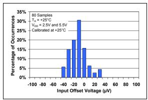
FIGURE 2-1: Input Offset Voltage.
