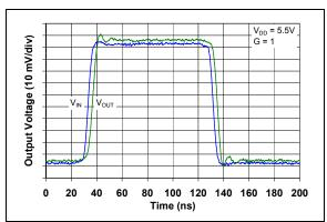
**FIGURE 2-37:** Non-inverting Small Signal Step Response.
