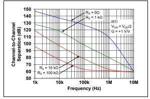
FIGURE 2-31: Channel-to-Channel Separation vs. Frequency.
