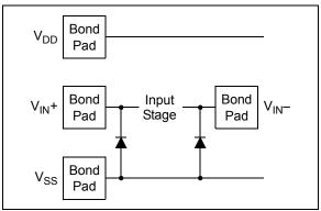
FIGURE 4-3: Simplified Analog Input ESD Structures.
