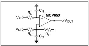
FIGURE 4-11: Amplifier with Parasitic Capacitance.
