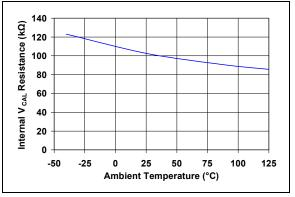
**FIGURE 2-23:** V<sub>CAL</sub> Input Resistance vs. Temperature.
