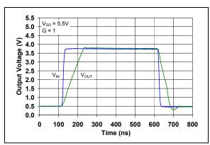
FIGURE 2-38: Non-inverting Large Signal Step Response.
