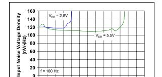
**FIGURE 2-33:** Input Noise Voltage Density vs. Input Common Mode Voltage with f = 100 Hz.
