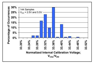
**FIGURE 2-22:** Normalized Internal Calibration Voltage.
