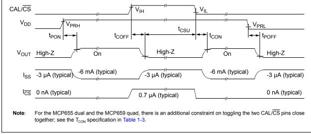
FIGURE 1-1: Timing Diagram.
