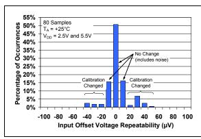
**FIGURE 2-3:** Input Offset Voltage Repeatability (repeated calibration).
