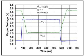
**FIGURE 2-40:** Inverting Large Signal Step Response.
