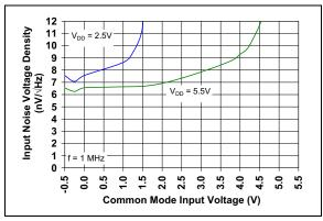
**FIGURE 2-34:** Input Noise Voltage Density vs. Input Common Mode Voltage with f = 1 MHz.
