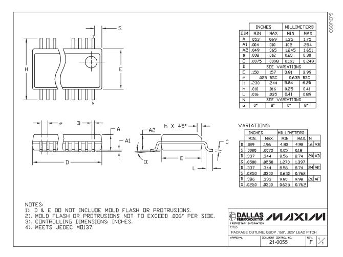
Note: The MAX1737EEI is a 28-pin QSOP and does not have a heat slug.
