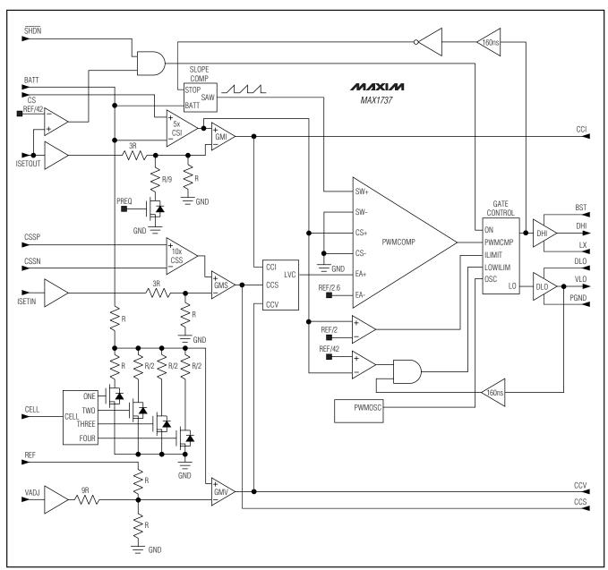
Figure 3. PWM Controller Block Diagram
