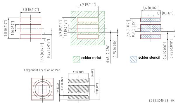
For superior solder joint connectivity results we recommend soldering under standard nitrogen atmosphere. Package not suitable for ultra sonic cleaning.
