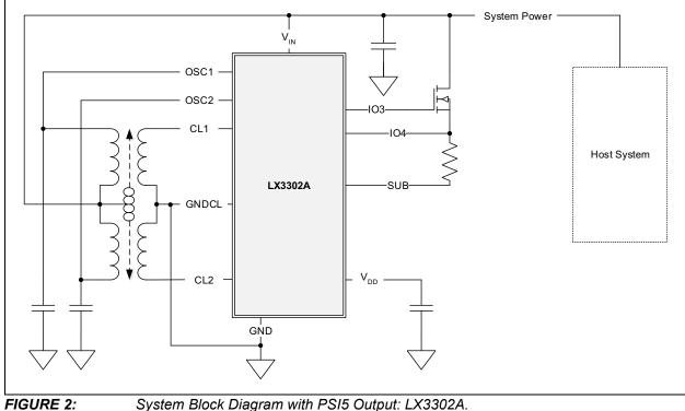
System Block Diagram with PSI5 Output: LX3302A.
