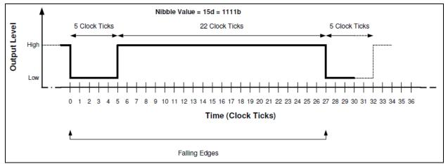
FIGURE 4-5: Timing Diagram for Nibble Value = 15d.
