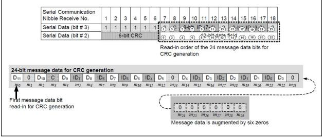
FIGURE 4-11: CRC for Enhanced Serial Message.
