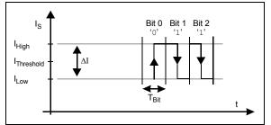
FIGURE 4-13: Bit Encoding by Current Modulation.
