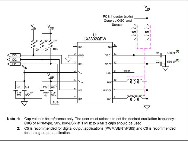
FIGURE 5-1: LX3302A 14-Pin Reference Schematic.
