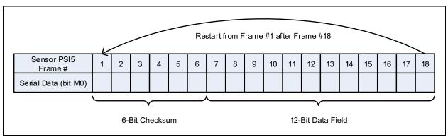
FIGURE 4-17: Serial Data Frame Generated by [M0] When M1[8] = 0.
