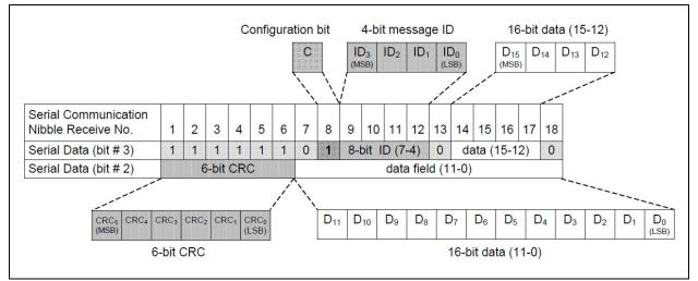
FIGURE 4-10: 16-Bit Data and 4-Bit Message ID.
