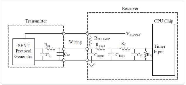
FIGURE 4-12: Example SENT Test Topology.
