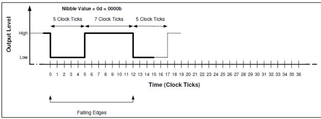
FIGURE 4-4: Timing Diagram for Nibble Value = 0d.
