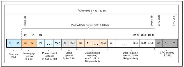
FIGURE 4-14: PSI5 Single Frame Sequence Format.
