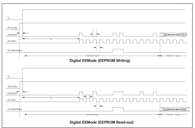
FIGURE 4-3: Digital EEPROM Timing Diagram.
