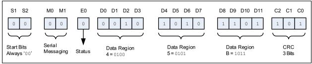
FIGURE 4-15: Encoded PSI5 Format for 0xB54.
