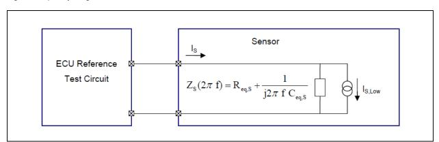
FIGURE 4-22: LX3302A Damping Behavior Model.
