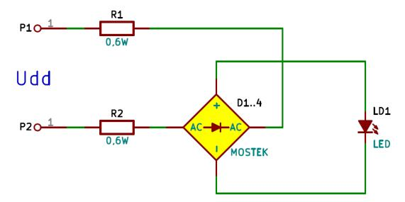
For 230V-AC voltage, power consumption is 0,5 W, for 24V-AC, it is 0,2 W and for 24V-DC, it is 0,5 W.
