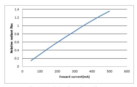
Fig 1. Relative Radiant Flux vs. Forward Current
