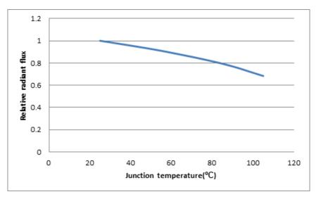
Fig.5 Relative Radiant Flux vs Junction Temperature
