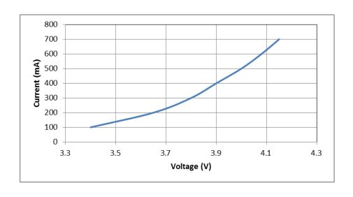
Fig 4. Forward Current vs. Forward Voltage
