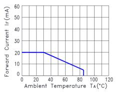
Fig.2 Forward Current Derating Curve
