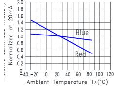
Fig.5 Relative Luminous Intensity VS. Ambient Temperature
