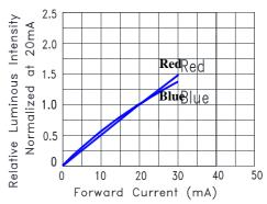
Fig.4 Relative Luminous Intensity vs. Forward Current
