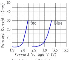
Fig.3 Forward Current vs. Forward Voltage
