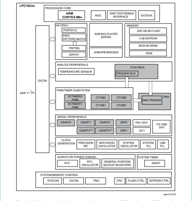
$Gray-shaded \ blocks \ show \ peripherals \ that \ can \ provide \ hardware \ triggers \ for \ DMA \ transfers \ or \ have \ DMA \ request \ lines.$
