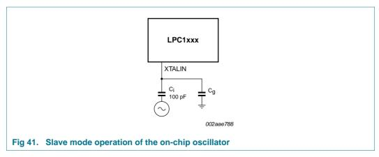
In slave mode the input clock signal should be coupled through a capacitor of 100 pF (Figure 41), with an amplitude between 200 mV (RMS) and 1000 mV (RMS). This corresponds to a square wave signal with a signal swing of between 280 mV and 1.4 V. The XTALOUT pin in this configuration can be left unconnected.
