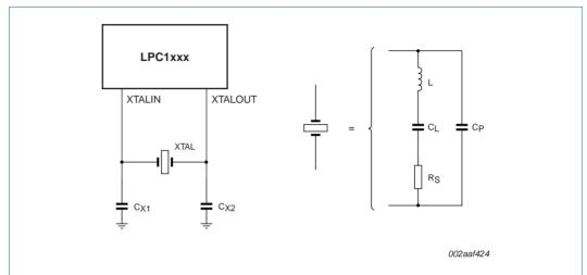
Fig 42. Oscillator modes and models: oscillation mode of operation and external crystal model used for  $C_{X1}/C_{X2}$  evaluation
