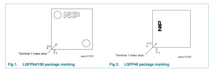
The LPC11U6x devices typically have the following top-side marking for LQFP100 packages:
