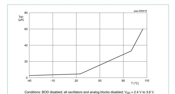
Fig 18. Power-down mode: Typical supply current  $I_{DD}$  versus temperature for different supply voltages  $V_{DD}$
