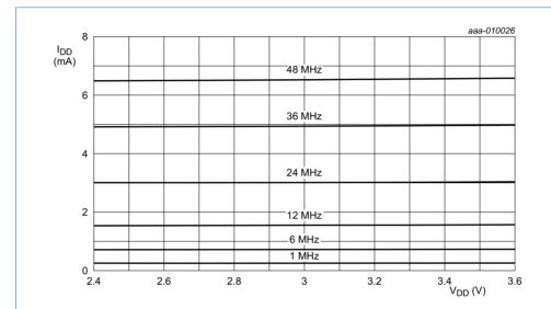
Conditions:  $T_{amb} = 25$  °C; active mode entered executing code while(1) {} from flash; all peripherals disabled in the SYSAHBCLKCTRL register (SYSAHBCLKCTRL = 0x1F), all peripheral clocks disabled; internal pull-up resistors disabled; BOD disabled; low-current mode.
