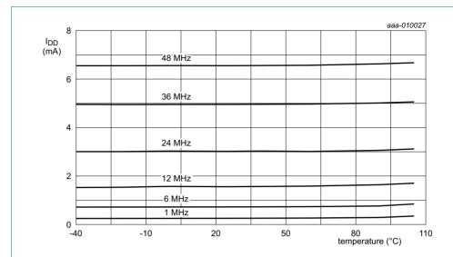
Conditions:  $V_{DD} = 3.3 \text{ V}$ ; active mode entered executing code while(1){} from flash; all peripherals disabled in the SYSAHBCLKCTRL register (SYSAHBCLKCTRL = 0x1F; all peripheral clocks disabled; internal pull-up resistors disabled; BOD disabled; low-current mode.
