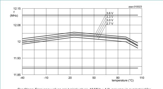
Conditions: Frequency values are typical values. 12 MHz  $\pm$  1 % accuracy is guaranteed for  $2.7~V \le V_{DD} \le 3.6~V$  and  $T_{amb}$  =  $-25~^{\circ}C$  to +85  $^{\circ}C$ . Variations between parts may cause the IRC to fall outside the 12 MHz  $\pm$  1 % accuracy specification for voltages below 2.7 V.
