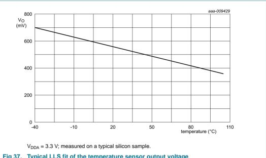
Fig 37. Typical LLS fit of the temperature sensor output voltage
