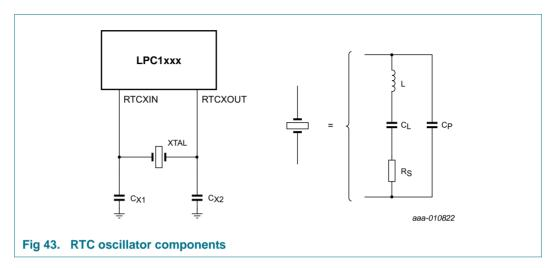
Select  $C_{x1}$  and  $C_{x2}$  based on the external 32 kHz crystal used in the application circuitry. The pad capacitance  $C_P$  of the RTCXIN and RTCXOUT pad is 3 pF. If the load capacitance of the external crystal is  $C_L$ , the optimal  $C_{x1}$  and  $C_{x2}$  can be selected as:
