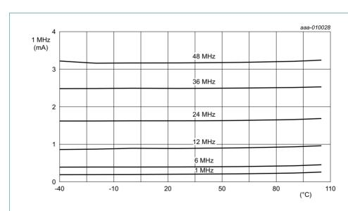
Conditions:  $V_{DD} = 3.3 \text{ V}$ ; sleep mode entered from flash; all peripherals disabled in the SYSAHBCLKCTRL register (SYSAHBCLKCTRL = 0x1F) all peripheral clocks disabled; internal pull-up resistors disabled; BOD disabled; low-current mode.
