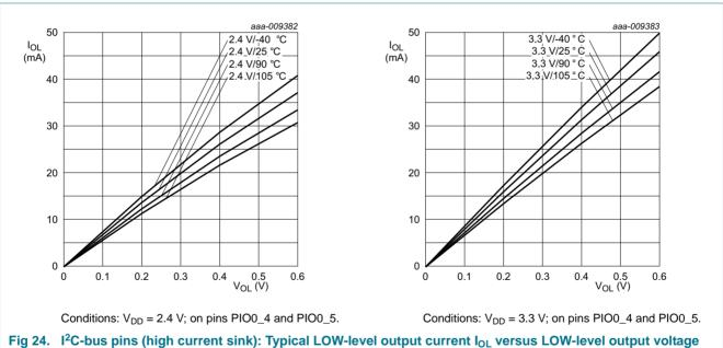
Fig 24. I<sup>2</sup>C-bus pins (high current sink): Typical LOW-level output current l<sub>OL</sub> versus LOW-level output voltage V<sub>OL</sub>
