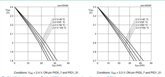
Fig 23. High-drive output: Typical HIGH-level output voltage V<sub>OH</sub> versus HIGH-level output current I<sub>OH</sub>
