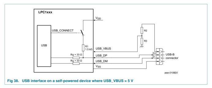
The USB\_CONNECT function can be enabled internally by setting the DCON bit in the DEVCMDSTAT register to prevent the USB from timing out when there is a significant delay between power-up and handling USB traffic. External circuitry is not required for the USB\_CONNECT functionality.
