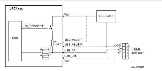
Two options exist for connecting VBUS to the USB VBUS pin:
