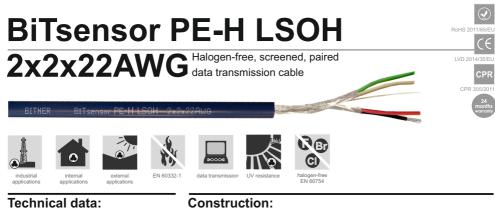
Operating temperature: -20°C to 80°C Min. installation temperature: -5°C Operating voltage: 300V Test voltage: 2500V Min. bending radius: 30mm
