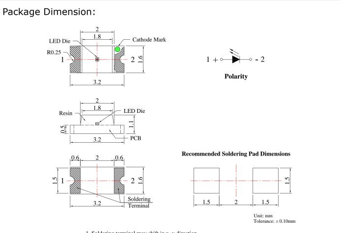
Soldering terminal may shift in x, y direction.
