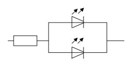
7.3 The pulse will destroy the fixed inner connection of LED, so the circuit must be designed carefully. When circuit open or close, LED will not be assaulted over-pressed (over-flow).
