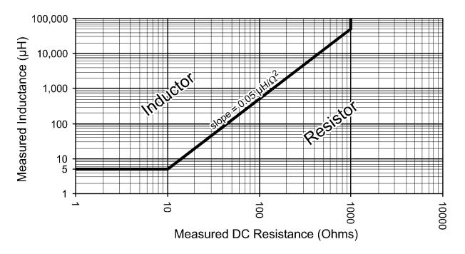
For example, if the inductance of your component is measured at  $100\mu$ H and it has a DC resistance of  $100\Omega$ , then the LCR45 will tell you that you have a resistor. If however the resistance was only  $10\Omega$ , then the LCR45 will tell you that you have an inductor.
