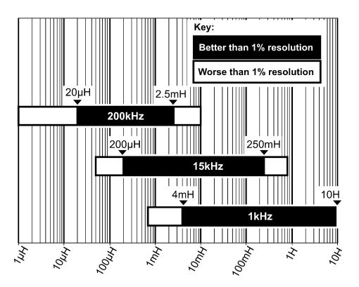
Measuring inductance outside of the black bands will result in degraded measurement resolution (possibly worse than 1% of the measured value).
