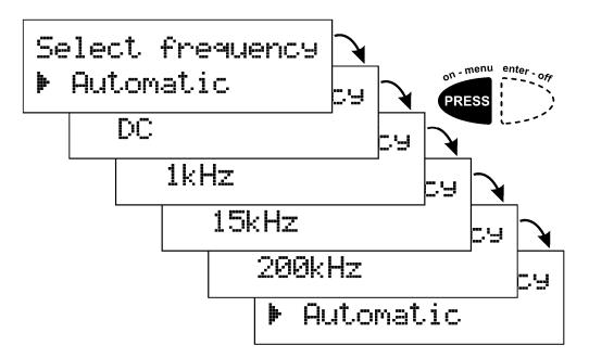
**Automatic** – The LCR45 will attempt to use the most appropriate test frequency to suit the component being tested. This is generally the best option for most requirements. It will automatically and dynamically select between DC, 1kHz, 15kHz and 200kHz.
