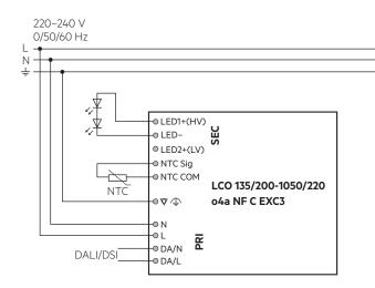
220-240 V 0/50/60 Hz L Ν ÷ ``{{ © LED1+(HV) SEC • LED-● LED2+(LV) - NTC Sig -• NTC COM LCO 135/200-1050/220 NTC o4a NF C EXC3 • 🌣 🛆 ΘN οL PRI ● DA/N DALI/DSI ● DA/L
