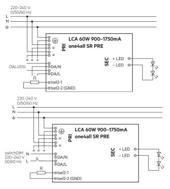
Device with loop through wiring function.
