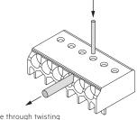
Loosen wire through twisting and pulling or using a Ø 1mm release tool
