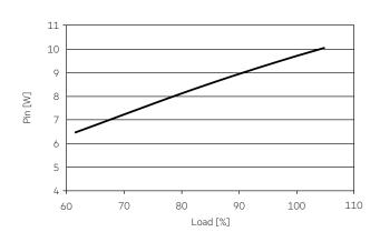
4.1.6 Phase cut dimming curve (depends dimmer)
