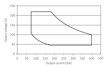
Make sure that the LED driver is operated within the given window under all operating conditions. Coming below the specified minimum output voltage of the LED driver may cause the device to shut-down.
