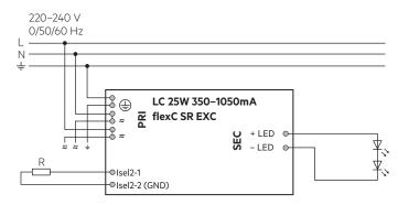
Device with loop through wiring function.
