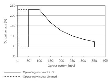
Make sure that the LED driver is operated within the given window under all operating conditions. Special attention needs to be paid at dimming and DC emergency operation as the forward voltage of the connected LED modules varies with the dimming level, due to the implemented amplitude dimming technology. Coming below the specified minimum output voltage of the LED driver may cause the device to shut-down. See chapter "6.11 DC operation" for more information.
