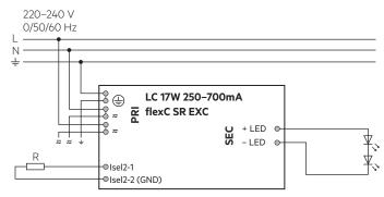
Device with loop through wiring function.
