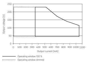
Make sure that the LED driver is operated within the given window under all operating conditions. Special attention needs to be paid at dimming and DC emergency operation as the forward voltage of the connected LED modules varies with the dimming level, due to the implemented amplitude dimming technology. Coming below the specified minimum output voltage of the LED driver may cause the device to shut-down. See chapter "6.9 DC operation" for more information.
