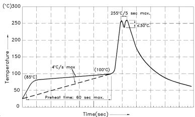
2.Peak wave soldering temperature between 245°C ~ 255°C for 3 sec (5 sec max).
