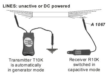
Fig. 16. Determination of individual wire
