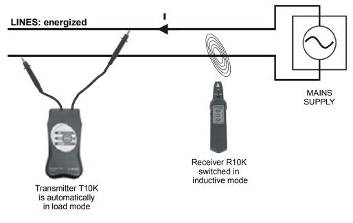
Fig. 3. Transmitter as active load
