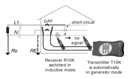
Fig. 15. Determination of short circuit location
