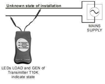
Fig. 11. Transmitter acts as energized state detector
