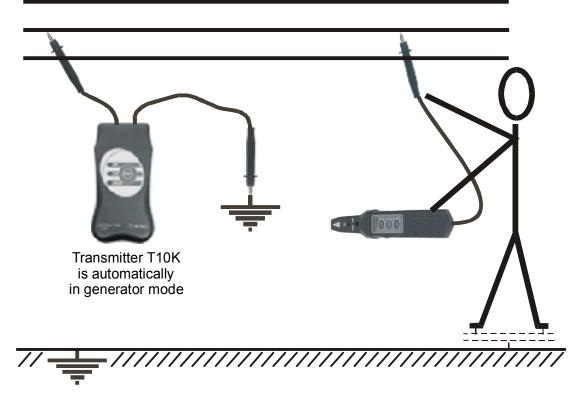
Fig. 10. Tracing the conductor using Test tip
