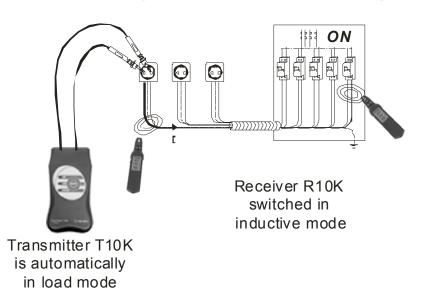
*Fig. 13.* Tracing cable or determination of the belonging fuse on energized installation. The receiver detects the electromagnetic field caused by load current of the transmitter.
