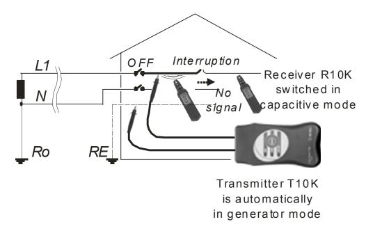
*Fig. 14.* Determination of interruption location-electrical field caused by transmitter disappears behind the interruption.
