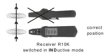
Fig. 4. Detection of electromagnetic field
