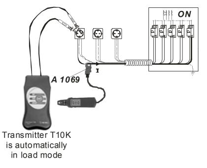
Fig. 17. Determination of the belonging fuse by using current clamp
