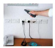
With various arrangements a detection depth between 40 and up to 200 cm can be reached on energized lines, a detection depth up to 40 cm can be reached on non-energized lines.
