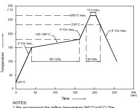
1.We recommend the reflow temperature 245° C(+/-5° C). The maximum soldering temperature should be limited to 260° C. 2 Don't cause stress to the epoxy resin while it is exposed
