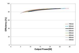
IT DALI 30 220 240 700 CS Typical Efficiency Vs Load 230V 50Hz
