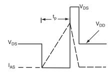
Fig. 12b - Unclamped Inductive Waveforms
