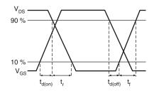
Fig. 10b - Switching Time Waveforms
