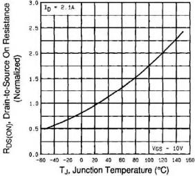
Fig. 4 - Normalized On-Resistance vs. Temperature
