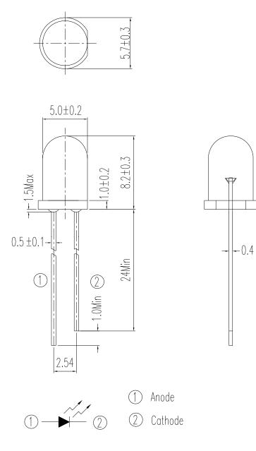
Note: Tolerances unless dimensions ±0.25mm
