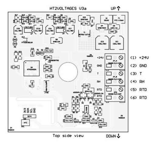
Figure 1. Outs Description of the HCRH-0x Series Sensor
