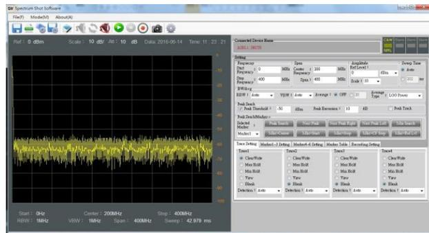
Under the Remote Control mode, users can monitor wireless interference signals or observe signals for long periods of time.
