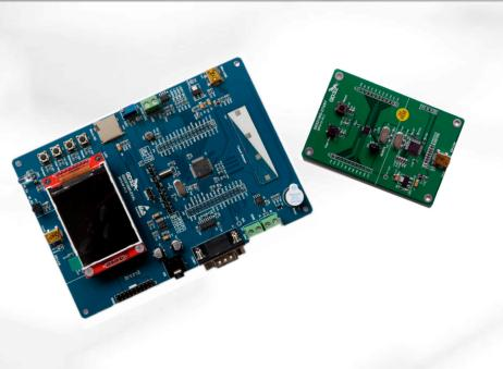
The Gigadevice Starter Kits include an I/O Extension Header for all of the package pins to allow quick connection of prototyping and probing. Also included on all of the boards is the GD-Link, a programmer and debugger for the GD32 MCU's.
