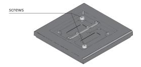
(3) Disconnect the button stand from the frame and electronics.
