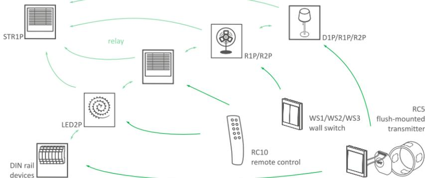
\* Range of up to 100 meters in open space without any interfering factors. In building conditions and in the presence of interference sources (power lines, transmitters, etc.) the actual range may be smaller.
