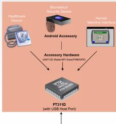
USB Connection providing data connectivity (Optionally, the Android Accessory can also charge the Android device)
