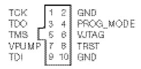
Pin 4 on FlashPro4 programmers must not be connected or used for other than their intended purpose.
