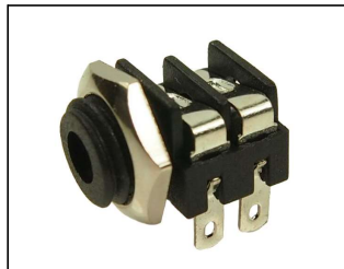
S6/BB mono switched 3.5mm Jack Socket. Panel mounting with solder tags. Also available with Special 'C' Contact to suit Far Eastern plugs. S6/BB (CL1382)
