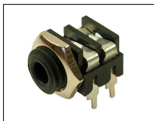
S6/BB PC mono switched 3.5mm Jack Socket. Right angle PCB mounting. Also available with Special 'C' Contact to suit Far Eastern plugs. S6/BB PC (CL1384)
