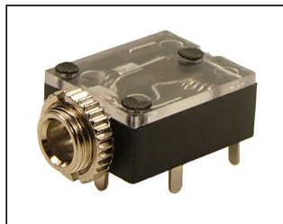
JYS-35 stereo switched 3.5mm Jack Socket. Right angle PCB mounting. Supplied with ring nut. JYS-35 (FT6320)
