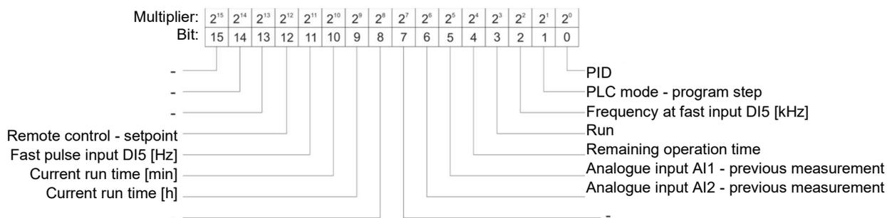
If any of the above-mentioned parameters is to be displayed while the drive is running, set the bit field corresponding to this parameter to 1. Next, convert the whole number to the hexadecimal (HEX) form, and write it to the **F6.02** in this form.
