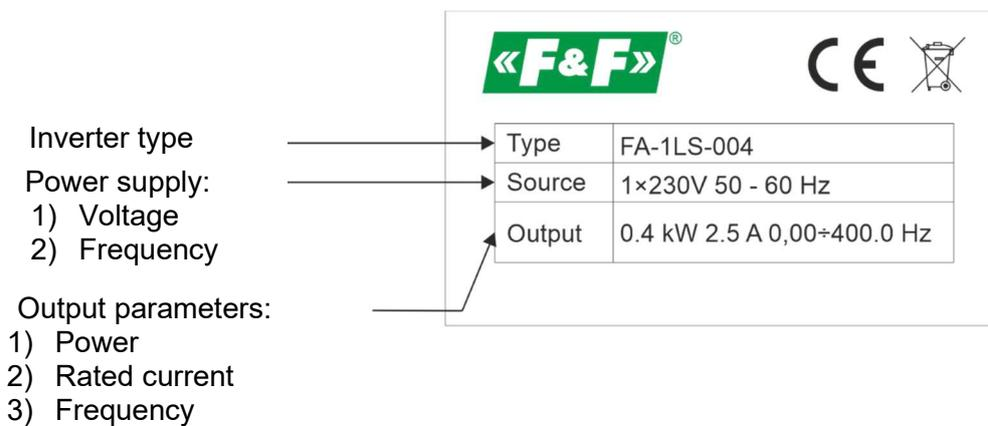
Fig. 1) Inverter nameplate
