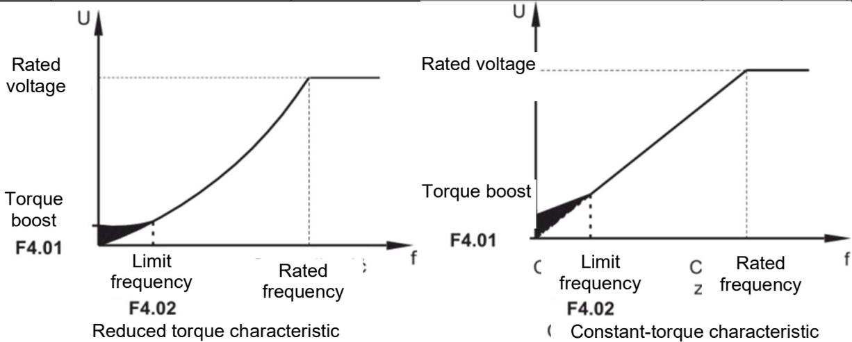
It is recommended that higher torque boost should be used for heavy drives where the standard drive torque is insufficient to accelerate them.
