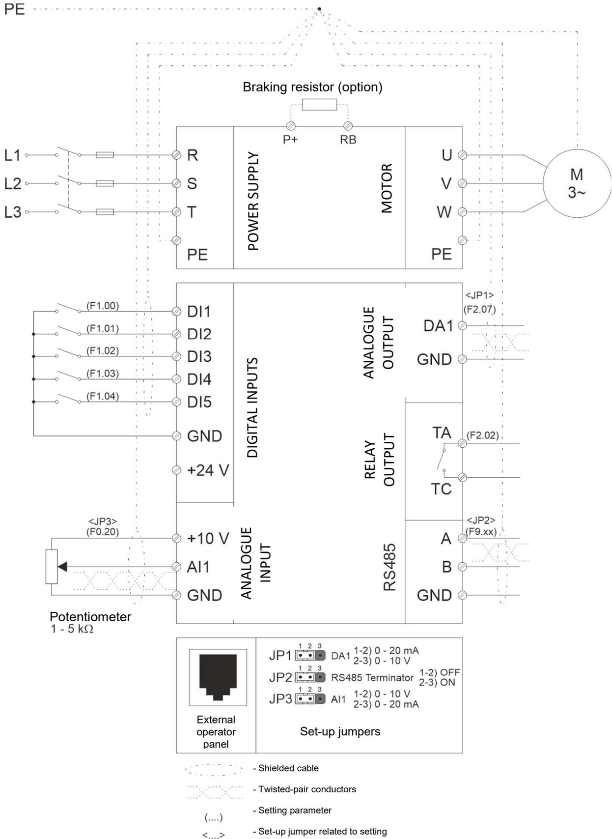
**Fig. 5) FA-3HS 3-phase inverter connection diagram**
