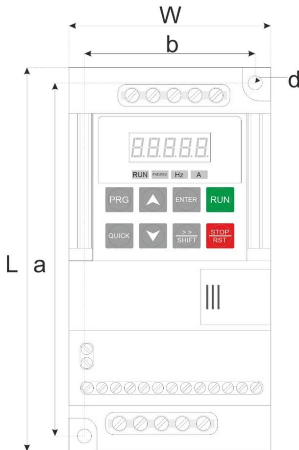
Fig. 12) Inverter dimensions and measurement hole locations
