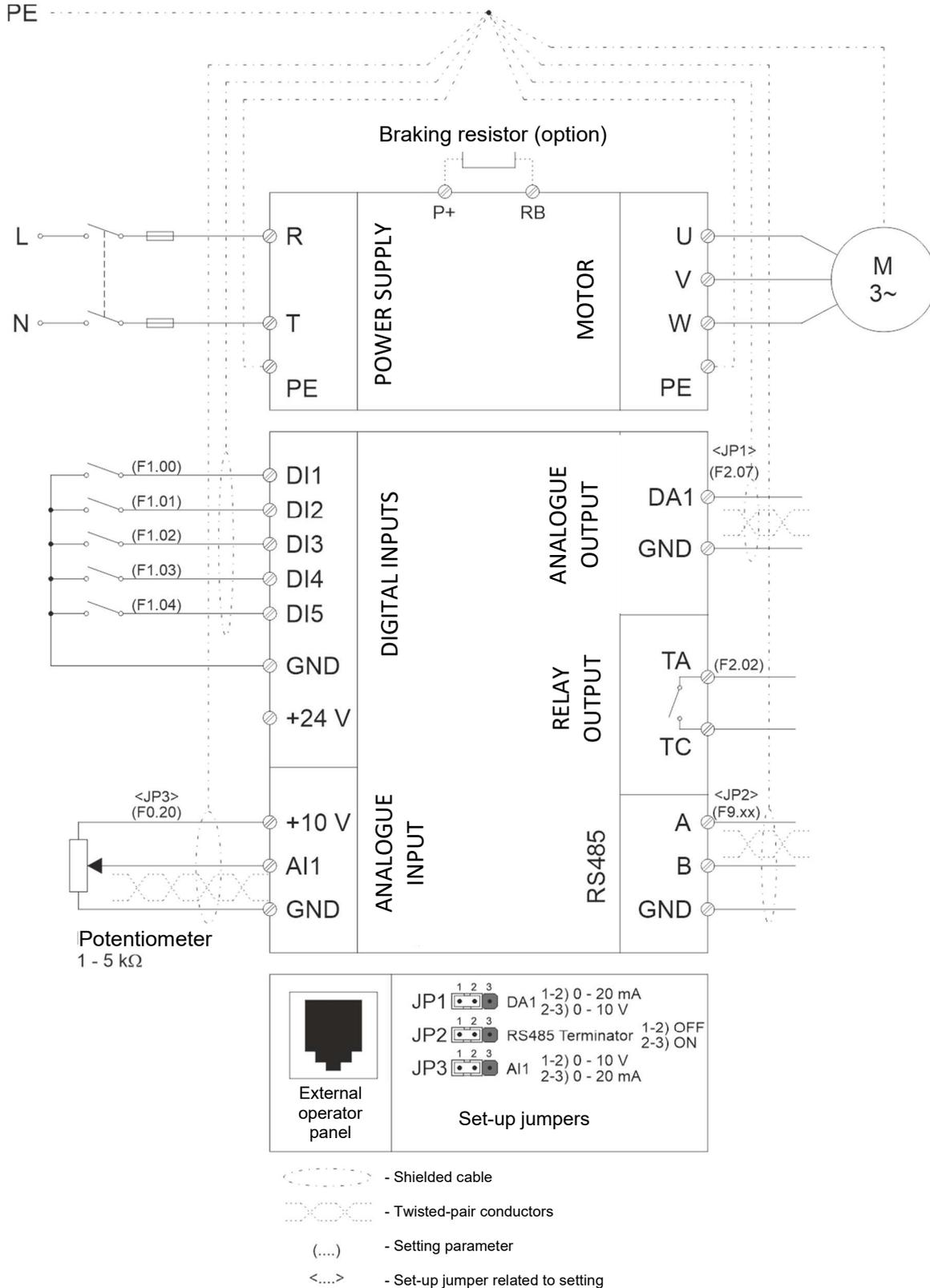
**Fig. 4) FA-1LS 1-phase inverter connection diagram**
