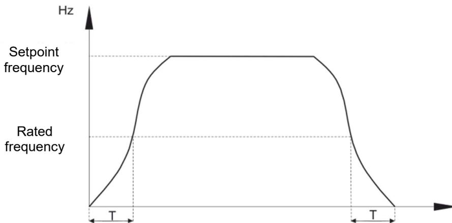
Acceleration/deceleration characteristic as per the second S-curve
