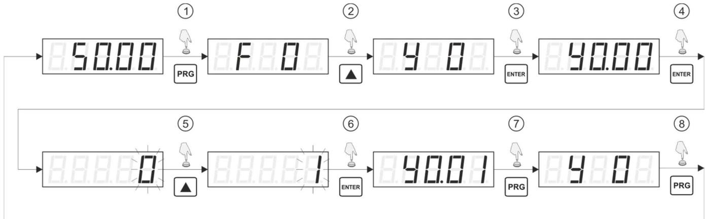
**Fig. 10) Procedure example - restoring the default set-up**
