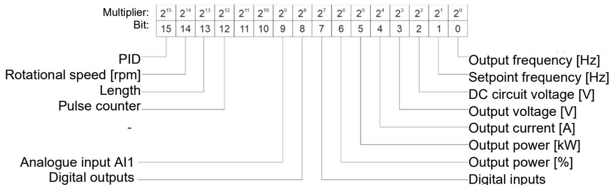
If any of the above-mentioned parameters is to be displayed while the drive is running, set the bit field corresponding to this parameter to 1. Next, convert the whole number to the hexadecimal (HEX) form, and write it to the **F6.01** in this form.
