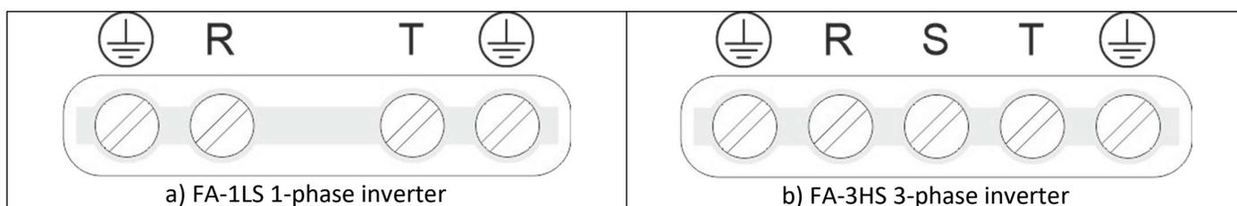
**Fig. 6) Inverter power supply connection terminal strip**
