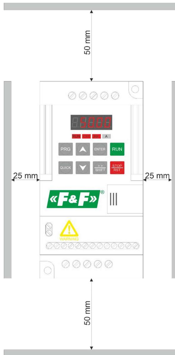
**Fig. 3) Correct inverter installation example**
