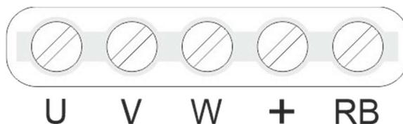
**Fig. 7) Motor connection**
