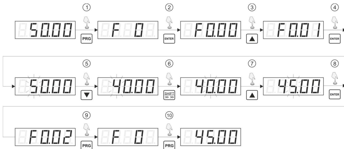
**Fig. 11 Procedure example – changing a setpoint**
