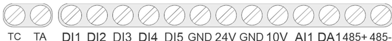
Fig. 8) Control circuit terminal strip
