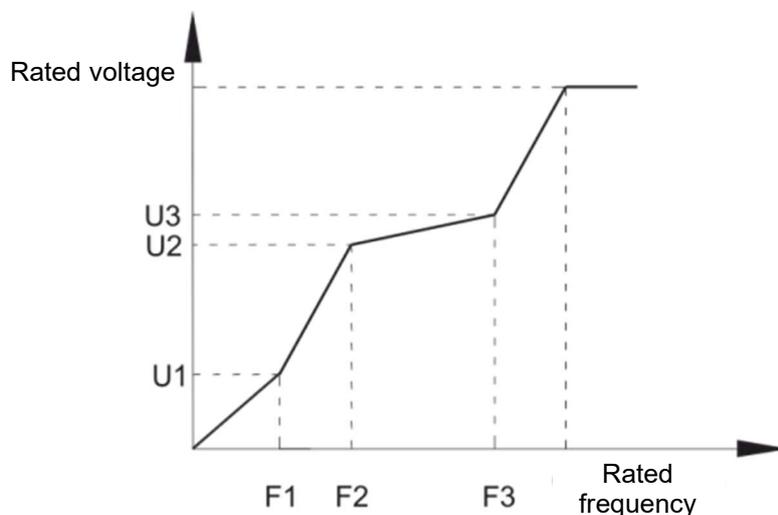
The following relationship between voltages and frequencies must be maintained while programming the U/f characteristic: **V1 < V2 < V3** and **F1 < F2 < F3**
