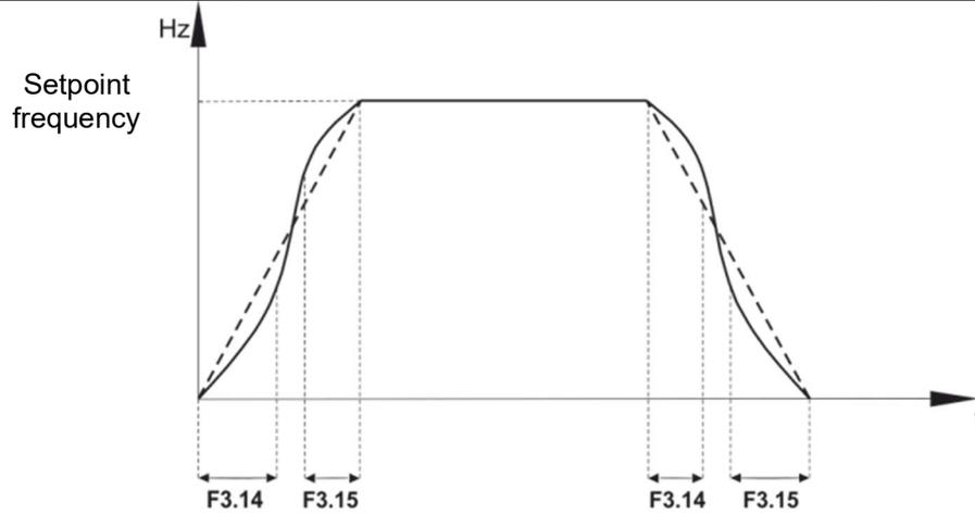
Acceleration/deceleration characteristic as per the first S-curve
