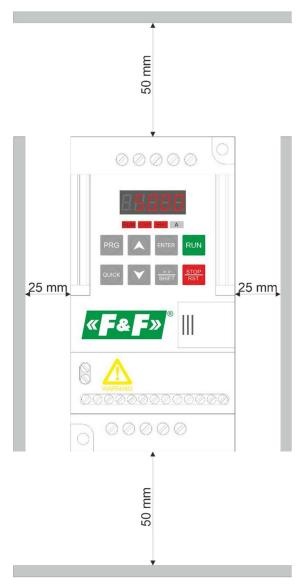
Fig. 3) Correct inverter installation example
