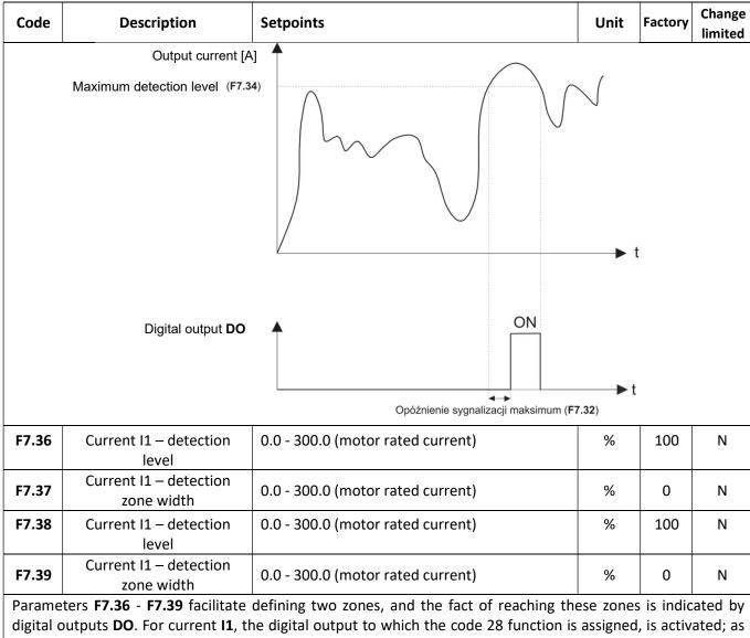
digital outputs **DO**. For current **I1**, the digital output to which the code 28 function is assigned, is activated; as for **I2**, the output to which the code 29 function is assigned, is activated. See the figure below for an operation diagram.
